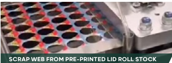
SCRAP WEB FROM PRE-PRINTED LID ROLL STOCK
